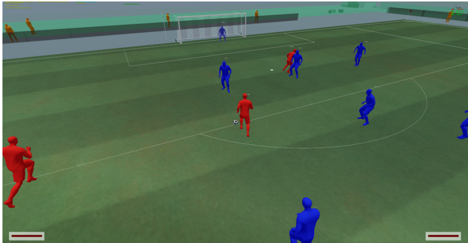
Figure 18: Example of a test in the automatic expert-authored test suite. In this test, the striker (in red, in the foreground) is threatening the center position of the goal net, and goalkeeper is very close to the goal line. In this type of situations, the goalkeeper should move forward. For this reason, in this situation the test checks whether the agent is moving towards the red striker.
