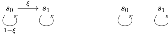
Figure 2: A two states, two actions Markov decision process used in example C.1 : the left and the right figures present the transition probabilities for actions a_0 and a_1 .
