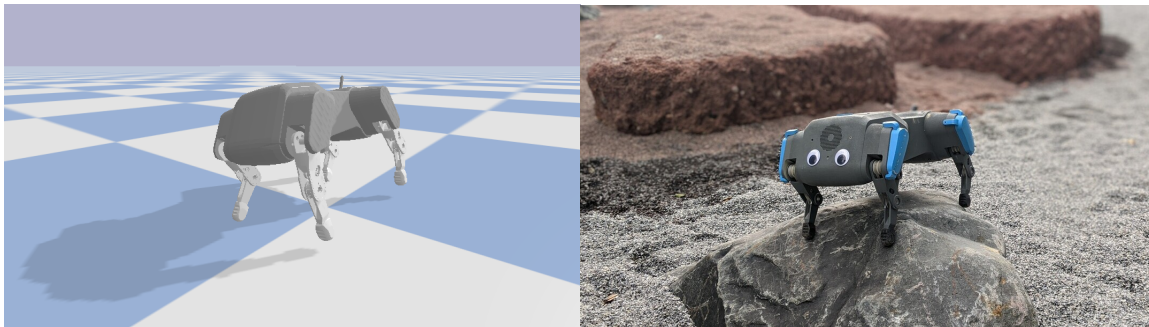
Figure 5: Robotic quadruped with elastic actuators in simulation (left) and real hardware (right)
